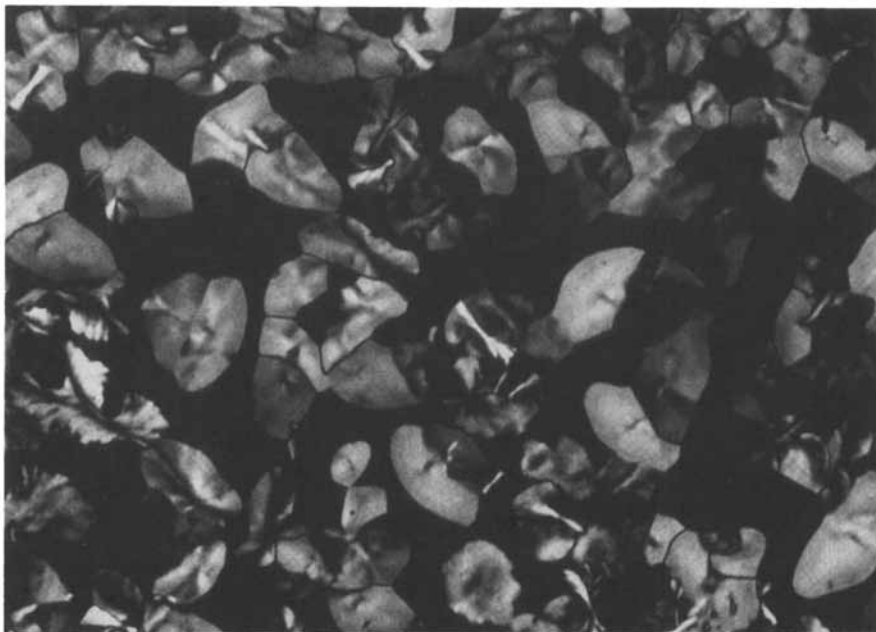
Figure 6. Polarized photomicrograph showing the formation of the mosaic structure in polymer HPX-C11 during a 0.5 K/min cooling scan from isotropic melt at 455 K.
