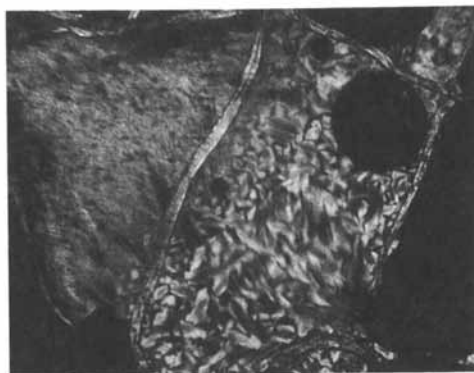
Figure 3. Coexistence of liquid crystalline and crystalline phases obtained on cooling of C_{12} diphosphate derivative.
